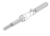
Fiber Optic Blocking Kit for Ribbon Fiber Cable, with central tube 11-15? mm OD
