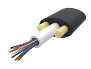
Fiber outdoor drop cable, LightScope® ZWP Self-Supporting All-Dielectric, Singlemode G.652.D and G.657.Al, 1–fiber Arid Core construction, Gel-filled, central loose tube, Feet jacket marking, Black jacket color
