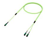
Ultra Low Loss (ULL) OM5, 1X2, MPO16 Multimode APC (Pinned) to MPO8 Multimode APC (Non-Pinned), 16-Fiber, Conversion Array, LSZH
