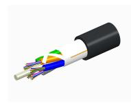
Fiber indoor/outdoor cable, LightSCOPE ZWP®, Single Jacket All-Dielectric, LSZH, 144 fiber, Gel-Free, Stranded Loose Tube, Singlemode G. 652.D and G.657.Al, Meters jacket marking, Black jacket color, Eca flame rating
