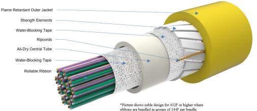
\*Picture shows cable design for 432F or higher where ribbons are bundled in groups of 144F per bundle. \*144F & 288F count designs use water blocking threads rather than a water blocking tape inside the buffer tube.
