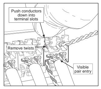
Figure 5. Seat Untwisted Pairs into IDC Terminal Slots
