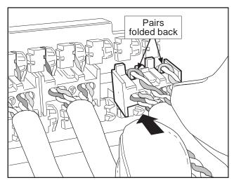
Figure 4. Snap Termination Manager onto Rear Housing
