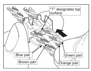
Figure 2. Feed Pairs into Termination Manager
