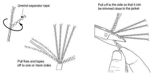
Preparation of the **SYSTIMAX GigaSPEED X10D 91B series cable**, **95B series cordage**, **or Xpress 88 series cable** is shown above. For complete instructions on preparing these cables for termination, see instruction sheet 860469402.
