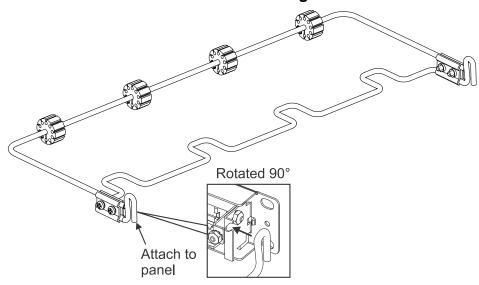
1. Attach fiber management bar to rear of panel immediately behind the fiber row. Place hook at both ends of bar into slots in panel brackets as shown.
