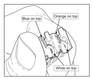
Figure 3. Fold Pairs Back into Slots
