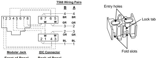
Front of Panel Back of Panel T568 Wiring Diagram
