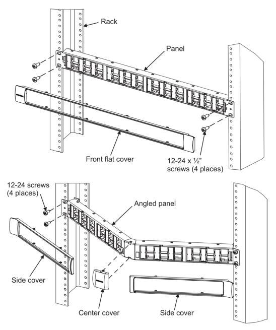
1. Mount panel to rack using the 12-24 screws provided. After securing the panel to the rack, snap the Evolve covers onto the front of the panel.
