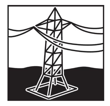
Do not install near power lines. Power lines, telephone lines, and guy wires look the same. Assume any wire or line can electrocute you. Do not install on a wet or windy day or when lightning or thunder is in the area. Do not use metal ladder.
