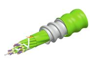
Fiber indoor cable, Riser/LSZH rated, MPO Trunk, interlocking aluminum armored, OM5 multi-mode, 128 fiber, Feet jacket marking, Lime gree jacket color, B2ca flame rating
