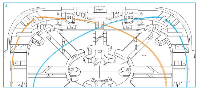
4 Overview of feeder fibers and branch fibers entering the top tray.
