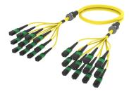
Singlemode MPO16 APC (pinned) to MPO16 APC (pinned), Fiber Trunk Cable Assembly, 192-Fiber, Armored Indoor Plenum
