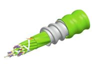
Fiber indoor cable, LazrSPEED® Plenum MPO Trunk, interlocking aluminum armored with plenum jacket, Multimode OM5, 32 fiber multiunit with 8 fiber subunits, Lime-green jacket color, Feet cable marking
