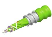
Fiber indoor cable, Plenum MPO Trunk, interlocking aluminum armored with plenum jacket, 192 fiber multi-unit with 16 fiber subunits, Gel-free, OM5 multi-mode, Feet jacket marking, Lime green jacket color
