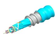
Fiber indoor cable, Plenum MPO Trunk, interlocking aluminum armored with plenum jacket, 128 fiber multi-unit with 16 fiber subunits, Gel-free, OM4 multi-mode, Feet jacket marking, Aqua jacket color
