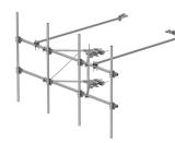
G22HDX Series High Capacity Three Sector Frame Kit for Towers, 12.5 ft x 2.88 in OD face pipes, includes twelve 96 in x 2.88 OD antenna pipes plus six 96 in RRU Pipes
