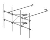
G22HD Series High Capacity Three Sector Frame Kit for Towers, 12.5 ft x 2.88 in OD face pipes, includes twelve 96 in x 2.38 OD antenna pipes plus six 96 in RRU Pipes
