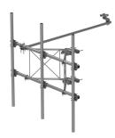
G21HD High Capacity Sector Frame, 10.5 ft 2.88 in OD face pipes, includes three 126 in 2.375 OD antenna pipes
