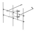
G23HDX High Capacity Sector Frame, 12.5 ft x 2.88 in OD face pipes, includes three 2.88 OD x 126 in antenna pipes.
