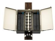
FDH5000 cabinet with 576 ports, LC/APC, no splitters, dry dielectric flat ribbon, 100 ft stub, 144F feeder, 288F distribution, pole mount
