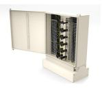
FDH5000 cabinet with 576 ports, LC/APC, no splitters, dry dielectric flat ribbon, 100 ft stub, 144F feeder, 288F distribution, pad mount with 8 in riser
