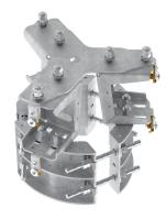
Pipe Mounting KIT with shroud, capability of mounting 37cm diameter round antennas (with trident mounting bracket, max length 2.1m, max weight 56kg) on the top of a pole with diameter from Ø150 to Ø273mm
