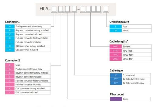
Cable length shown as an example; additional cable lengths available upon request up to 2,000 ft (600 m)
