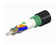
Fiber OSP cable, LightScope ZWP® Single Jacket/Single Armor, 144 fiber, Gel-Free, Stranded Loose Tube, Singlemode G.652.D and G.657.A1, Feet jacket marking, Black jacket color
