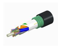
Fiber OSP cable, LazrSPEED® Single Jacket/Single Armor, Gel-Free, Stranded Loose Tube, 12 fibers, Multimode OM3, Feet jacket marking, Black jacket color
