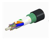
Fiber OSP cable, LazrSPEED® Single Jacket/Single Armor, 48 fibers, Gel-Free, Stranded Loose Tube, Multimode OM3, Feet jacket marking, Black jacket color
