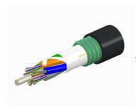
Fiber OSP cable, LazrSPEED® Single Jacket/Single Armor, 144 fiber, Gel-Free, Stranded Loose Tube, Multimode OM4, Feet jacket marking, Black jacket color
