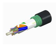
Fiber OSP cable, LazrSPEED® Single Jacket/Single Armor, 288 fiber, Gel-Free, Stranded Loose Tube, Multimode OM4, Feet jacket marking, Black jacket color
