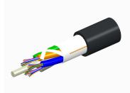
Fiber OSP cable, TeraSPEED® Single Jacket All-Dielectric, Gel-Free, Stranded Loose Tube, 24 fibers, Singlemode G.652.D and G.657.A1, Feet jacket marking, Black jacket color
