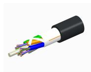
Fiber OSP cable, TeraSPEED® Single Jacket All-Dielectric, 96 fiber, Gel-Free, Stranded Loose Tube, Singlemode G.652.D and G.657.Al, Feet jacket marking, Black jacket color
